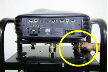
b) the image centers are horizontally shifted: act on the left adjustment wheel (see below images) to shift horizontally the upper projector respect the below one that will be used as reference.
