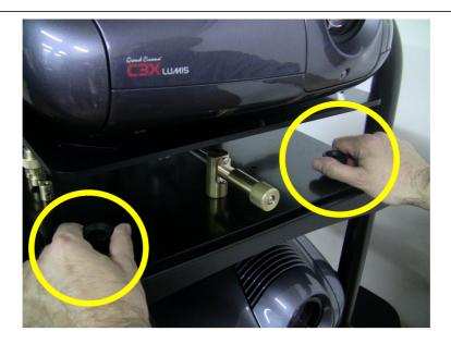
5. The images could be horizontally tilted one respect to each other, the image centers are horizontally shifted and the image dimensions slightly different.
