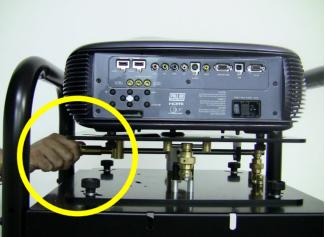
c) Following the instructions at points a) and b) you should have found the common image center. Now you could see that the image sides are not perfectly coincident. It means that the two images have slightly different zoom. Act on the front adjustment wheel to fine zooming the projector forth or back depending on the error you notice on the screen.
